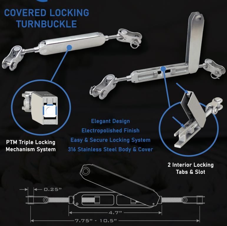
316 Stainless Steel Working Load: 1000 lbs Breaking Load: 2800 lbs Weight: 0.44 lbs
